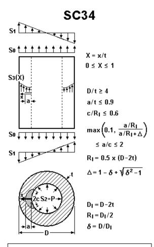
Notes: Internal pressure (S2) implies that the cylinder is capped and generates an additional axial stress.
